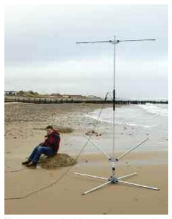
$\ensuremath{\mathsf{DX}}$  on the water's edge - the whole antenna is very light and can be moved around easily.
